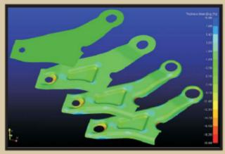
Iterate on intermediate geometries, blank size, blank position, and forming conditions for different stamping operations
